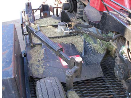
Figure 3-1. Mowing clippings completely covering mower decks
