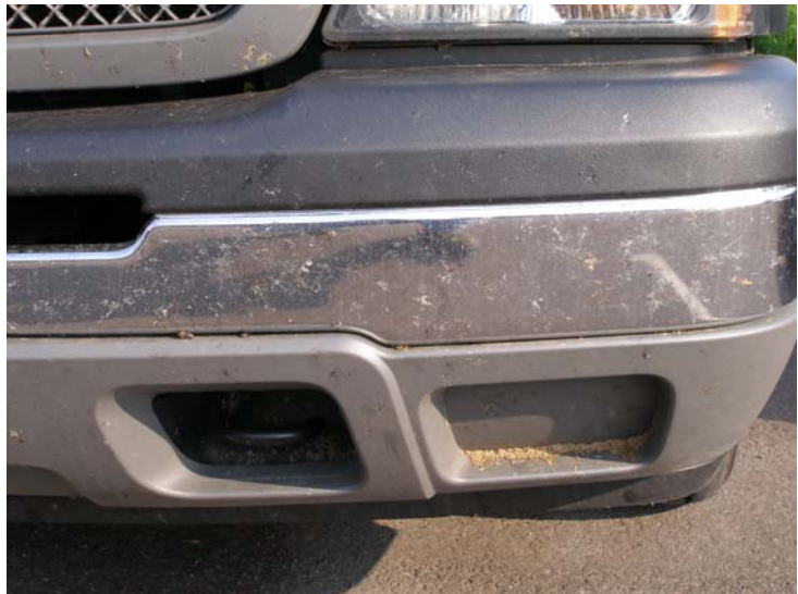
Figure 3-2. Seeds lodged in vehicle light reservoir
