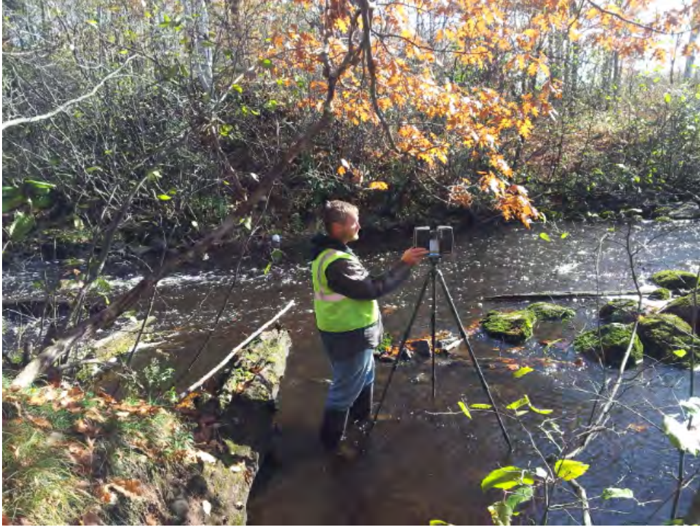
Figure 56. Laser scanning at the Tamarack Creek dam site in Pine County.
