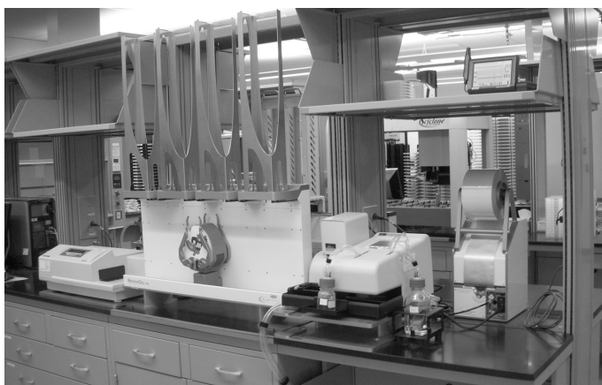
Integrated laboratory HTS automation system for conducting assays in microplates at the ITDD.
