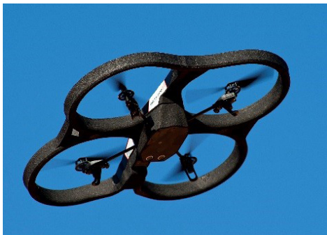
Fig. 1: Multicopter UAS equipped with multiple rotating propellers
