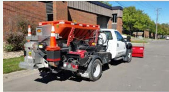
**Implementation:** Before a snow event, staff hook up the flatbed hook body to a one-ton truck using the SwapLoader system. When a request comes in, staff are able to drive directly to the request location and use the necessary tools and equipment from the flatbed.
