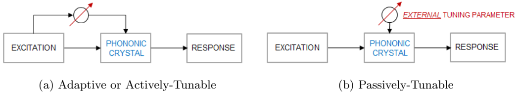
Figure 1.9: Schematic of structural logic for active and passive tuning of spectro-spatial characteristics of nonlinear periodic structures.
