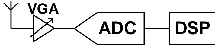
Figure 2.1: Single ADC based receiver
