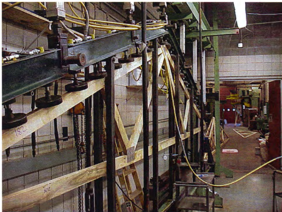
Figure 5.--Hardwood pitched chord truss during full scale testing.
