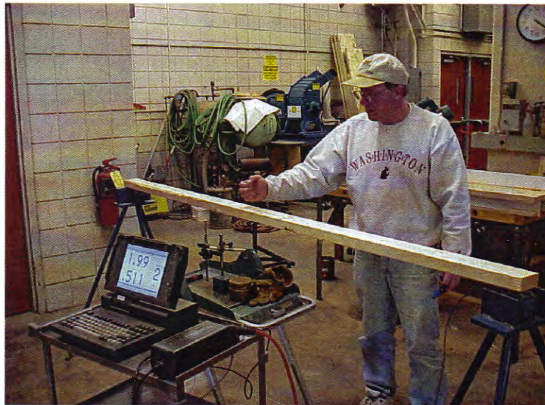
Figure 1.--Grading hardwood lumber using a commercial E-computer.
