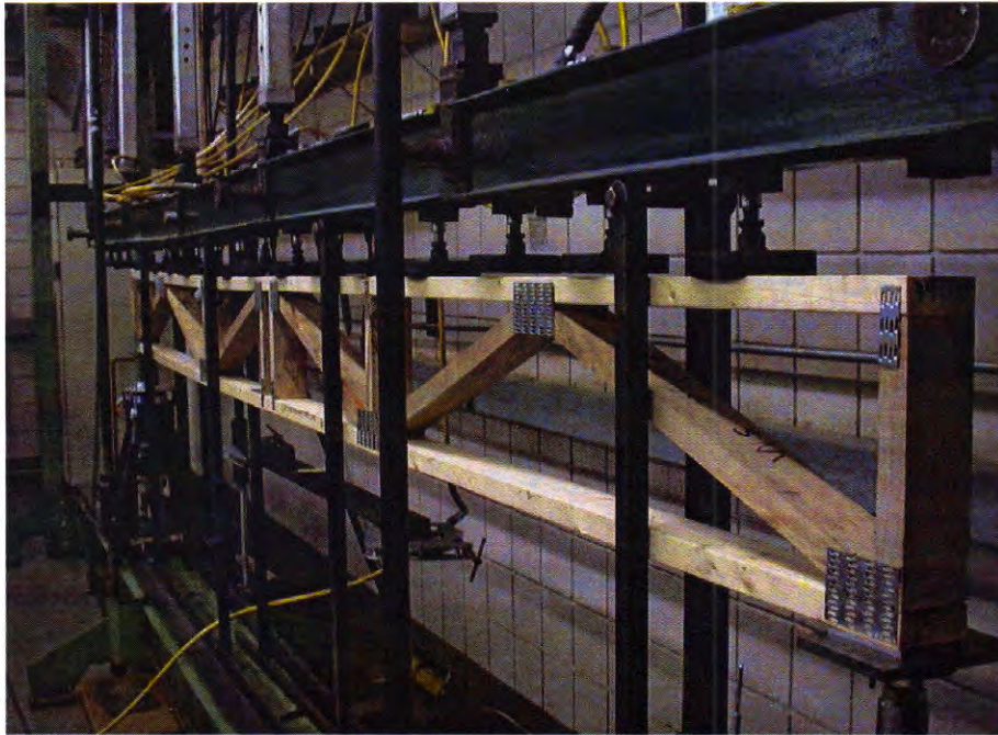
Figure 6.--Parallel chord truss testing setup.
