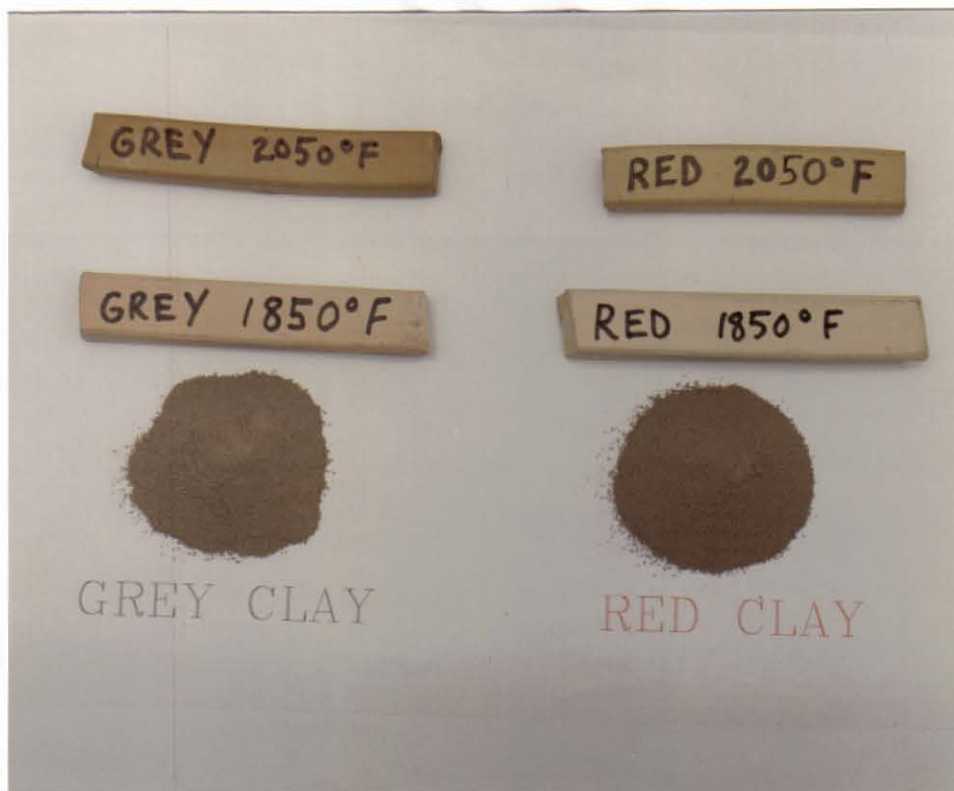
Plate 1. Raw clays and fired test bricks shown above are examples which depict the shift in the color of the clays as firing temperatures increase.
