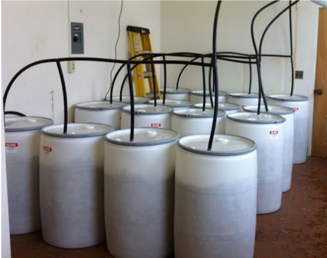
Figure 14. Sealed, vented inoculum tanks culturing sulfate-reducing bacteria sampled from stream sediment near the pit lake site.
