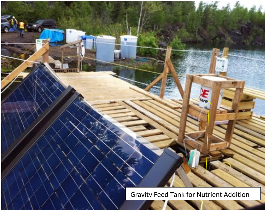
Figure 15. Bioreactor nutrient addition design.
