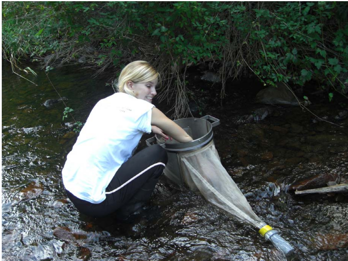
Photo 3. Undergraduate field assistant Kelia Axler collecting macroinvertebrates using a Hess sampler.
