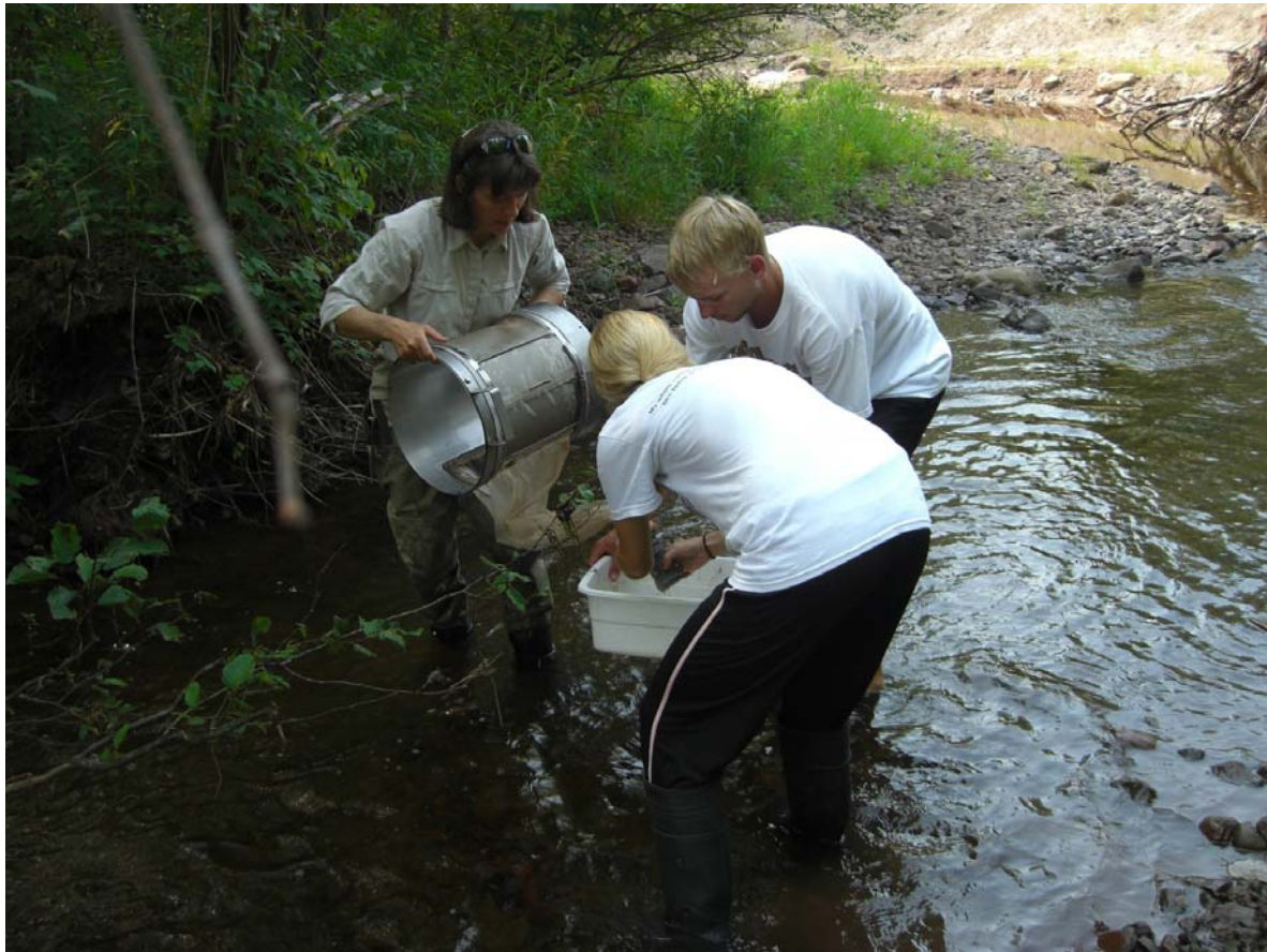
Photo 4. PI Valerie Brady (left) and field assistants Kelia Axler and Cory Peterson wash macroinvertebrates out of a Hess sampler and into a collection basin in preparation for preservation. Site is Amity Creek.
