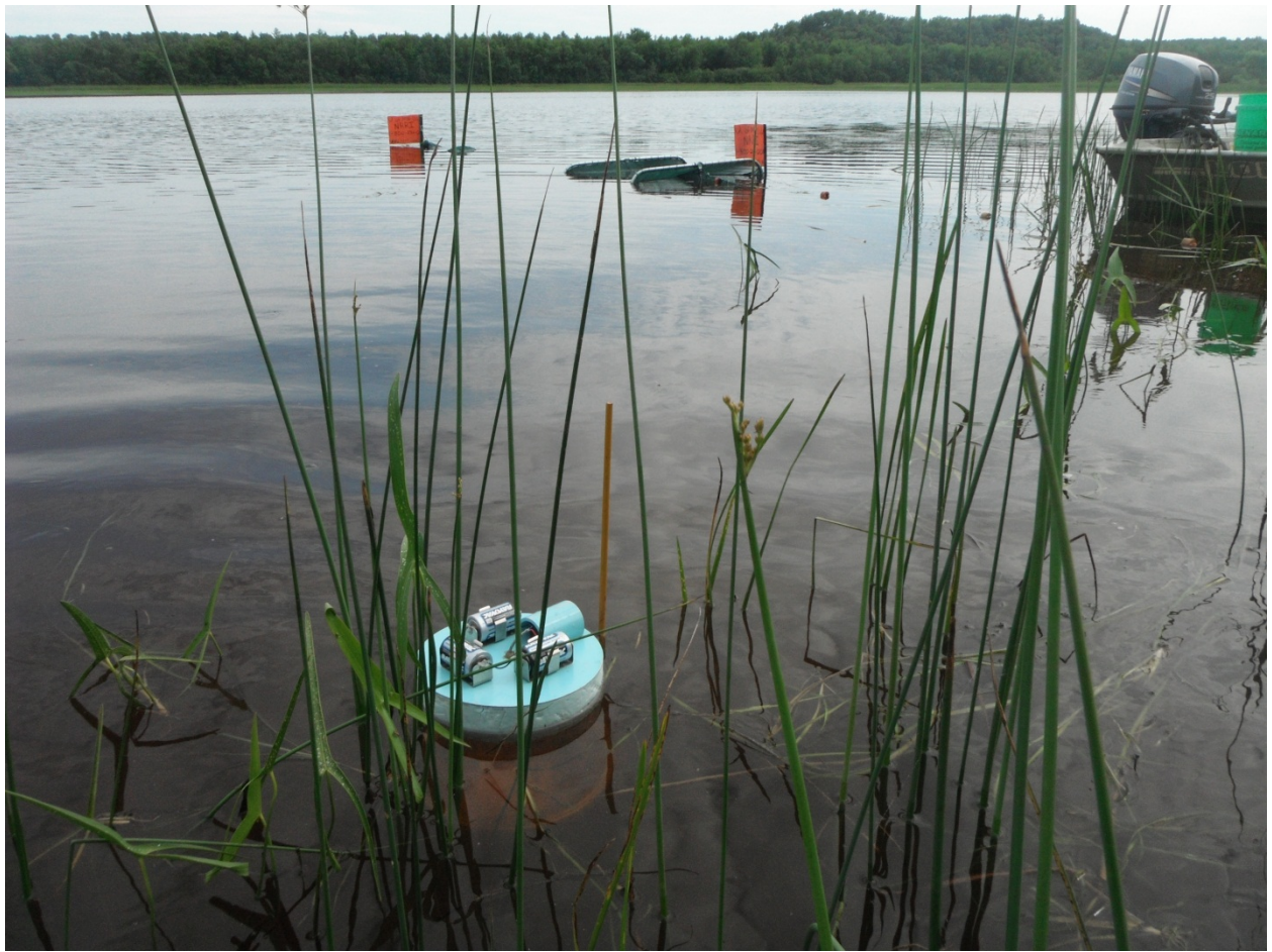
Figure 15. A larval trap set in Radio Tower Bay during the 7/29/2011 sample event. Larval traps were set near aquatic vegetation edges and close to fyke net locations.
