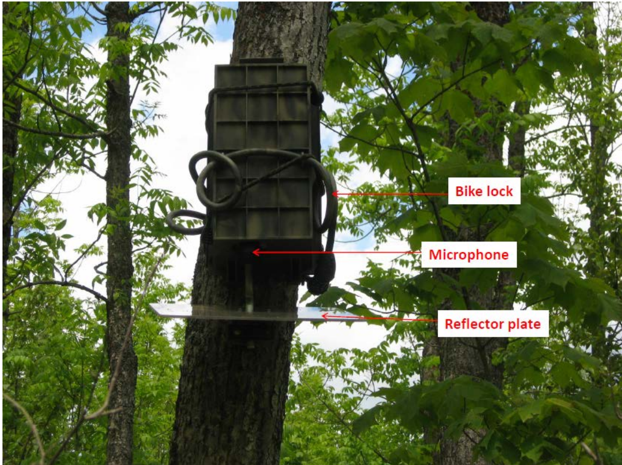
Figure 1.1. Weather-proof container designed to house the Anabat II bat detector system with a 12-volt battery for three nights. June, 2009. Taken by Becky Abel.
