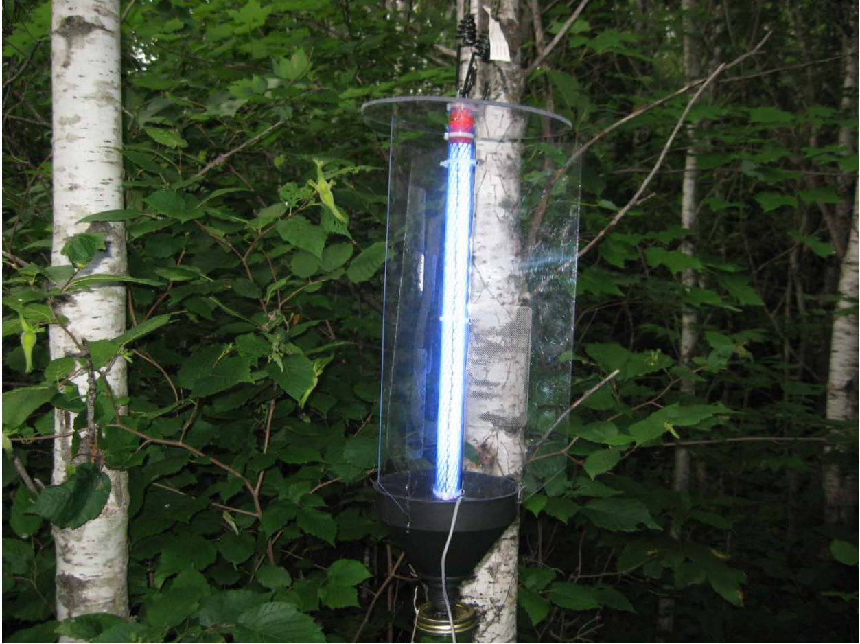
Figure 1.5. Insect black light trap near a bat detector site. Most insects are attracted to ultra-violet light and become trapped after hitting the clear plastic baffles and falling into the funnel and jar pictured at the bottom. July, 2009. Taken by Becky Abel.
