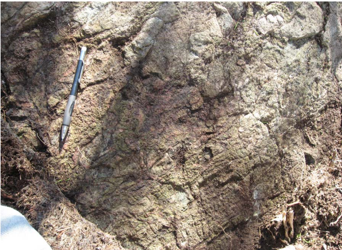
Figure 8. Strong epidotization (both pink and green epidote) commonly exhibited by the Altered Unit (OC-004W: UTM = 565,169E; 5,299,569N).
