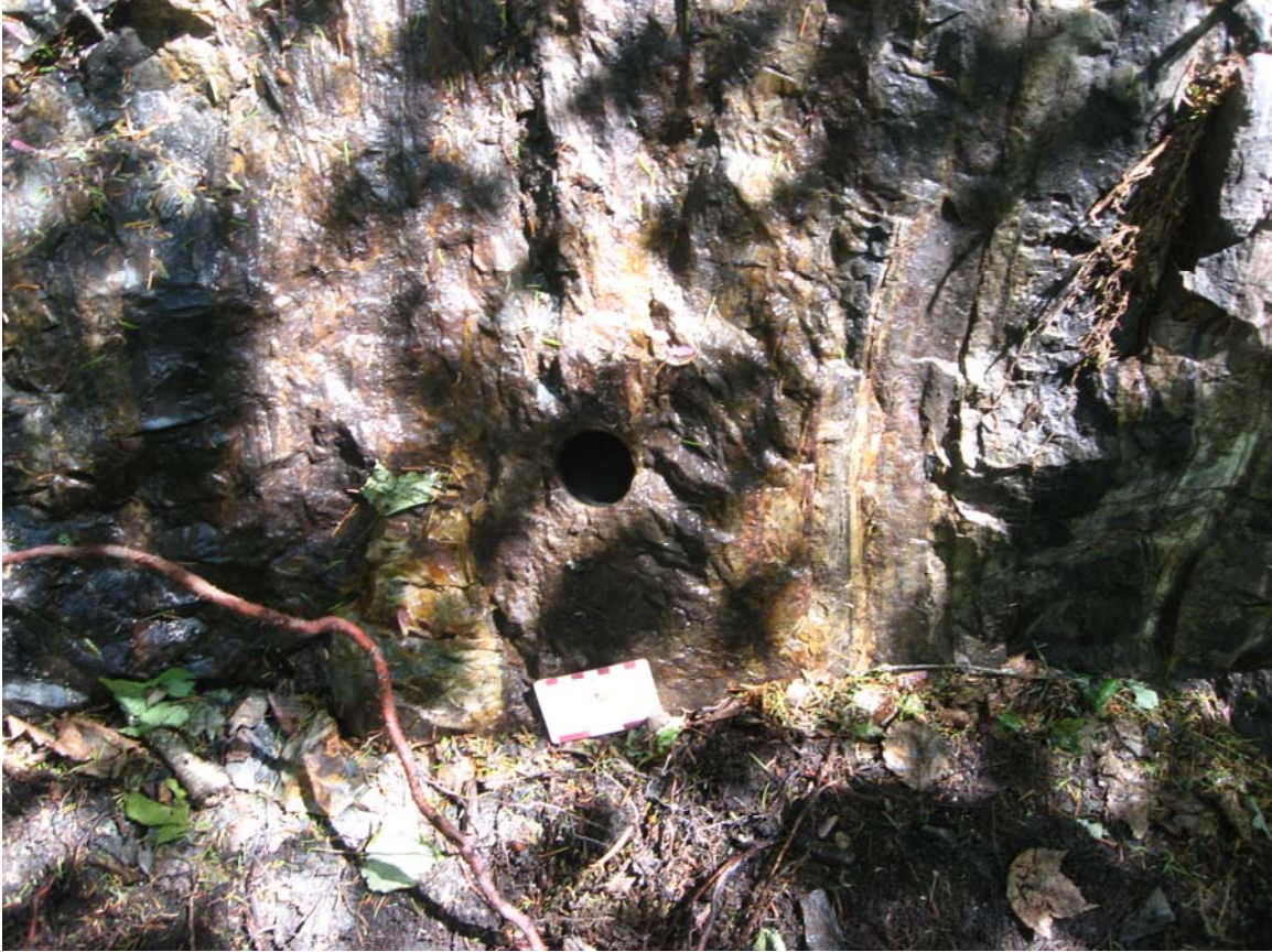
Figure 26. Drilled portion of gossan-coated Soudan Iron-formation at sample site OC-030 (UTM = 563,131E; 5,298,800N). No sulfides were seen in the four-inch long cored segment obtained at this site. Note that bedding is vertical and can be seen on the right side of the photograph.
