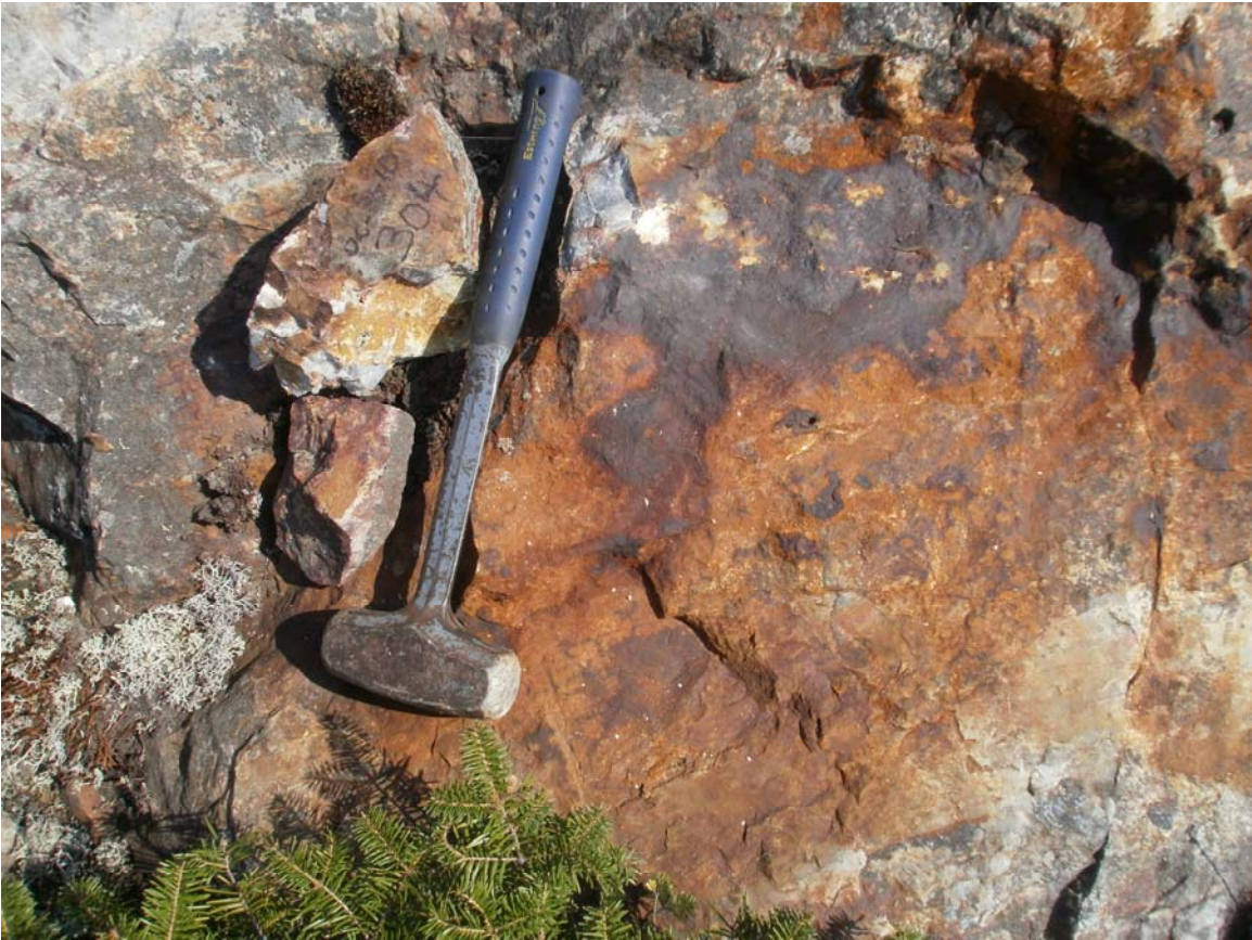
Figure 17. Presentation of iron-staining associated with disseminated pyrite in a chert band near the top of the Soudan Iron-formation at sample site OC-304 (UTM = 563,391E; 5,299,329N) with visually estimated 3% pyrite. This sample site is just north of present Highway 169 and near the west end of the proposed North Route. Similar material is also present in nearby drill holes. Overall, this type of sulfide-bearing material is presumed to be locally present in portions of the wetlands beneath the proposed corridor for the North Route.
