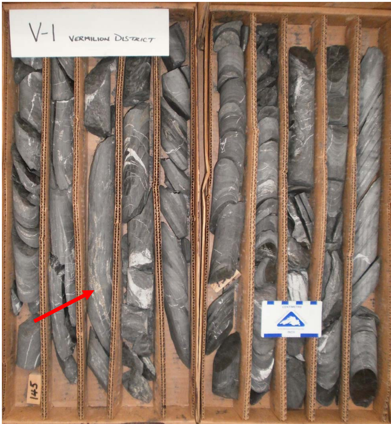
Figure 43. Drill core of a pyrite-bearing Graphitic Argillite unit, within the Gafvert Lake volcanoclastic unit, as intersected in drill hole V-1 at 145-164 feet. This unit is well-bedded (note the angle at which the core breaks), and contains bedding-parallel and cross-cutting quartz veins (white bands). Most of the pyrite is associated with the quartz veins, and it averages about 5% of the rock with localized high concentrations as high as 15% visually-estimated pyrite (note the red arrow).
