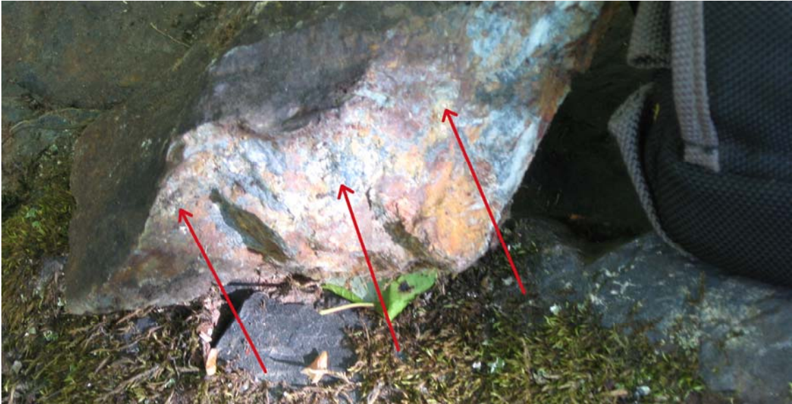
Figure 22. Coarse-grained massive pyrite aggregates, and intense iron-stained halos, associated with garnet-rich Soudan Iron-formation at sample site OC-49B (UTM = 563,781E; 5,299,102N). This sample contains approximately 15% visually estimated pyrite, and is located about 90 feet to the north of the centerline of the proposed South Route.
