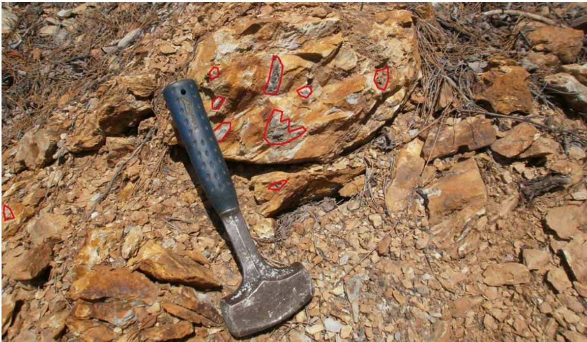
Figure 23. Discontinuous massive sulfide patches up to a few centimeters across in intensely sulfide-stained and moderately-sheared tuffaceous sediments of the Gafvert Lake volcanoclastic unit at sample site OC-091 (UTM = 563,413E; 5,299,586N). These rocks contain approximately 10% visually estimated pyrite and are located well to the north of the centerline of the proposed North Route (about 940 feet north). This outcrop was exposed in a relatively new borrow-pit along the edge of a major east-west trending swamp. The “swamp-edge” location of this exposure, and easily-weathered nature of the rock type, indicates that portions of the wetlands along the North Route corridor could be underlain by similar materials.
