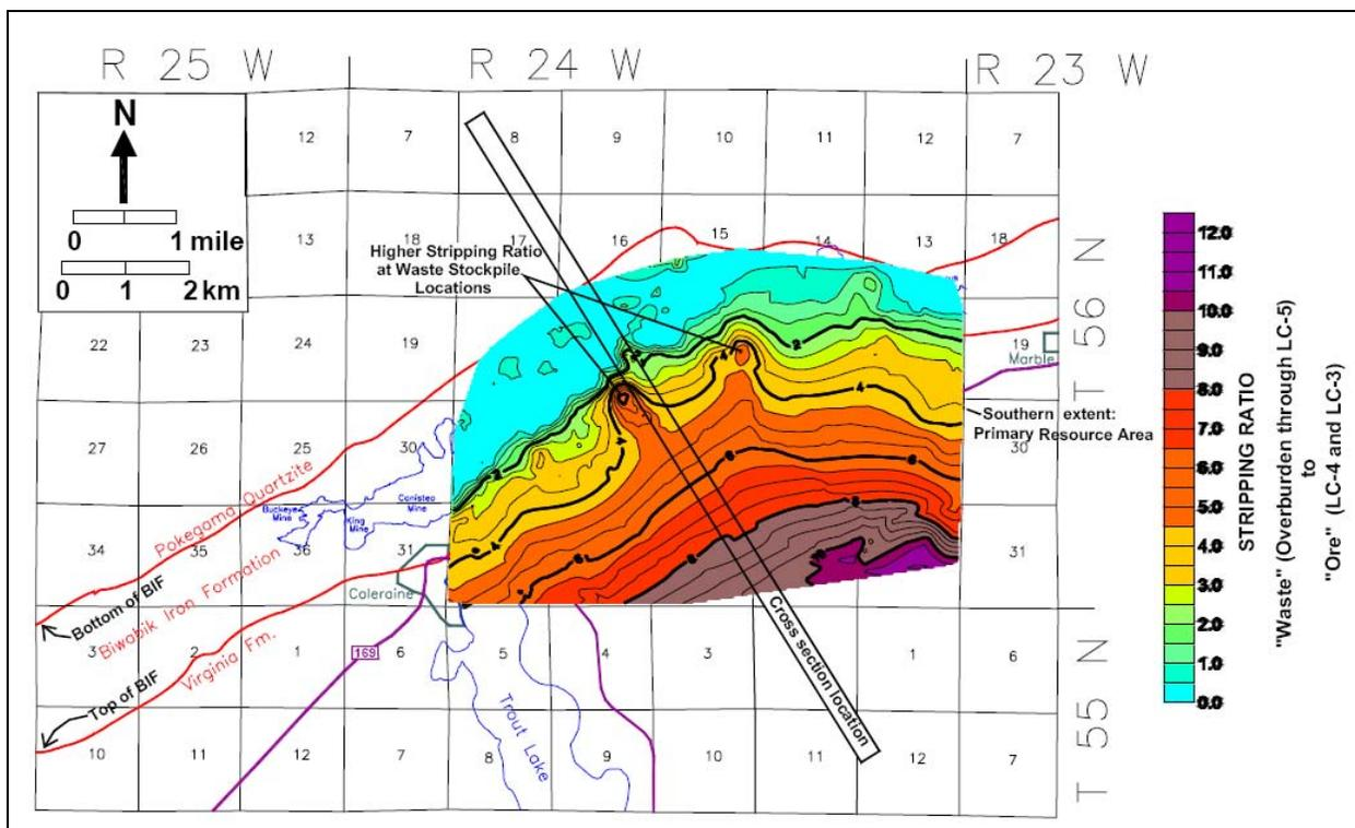
**Figure 1.** "Waste" (overburden through LC-5) to "Ore" (LC-4 and LC-3) ratio (stripping ratio) within area of interest (Zanko et al., 2003).
