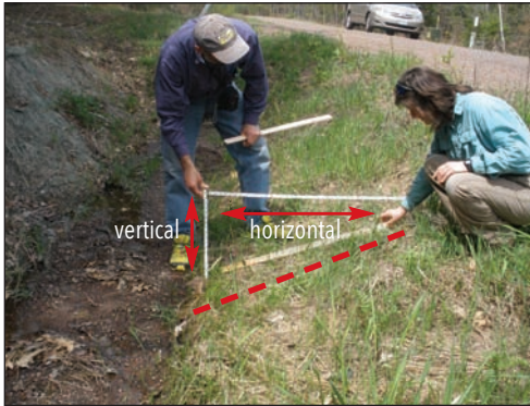
Figure 42: Ditch front slope example
