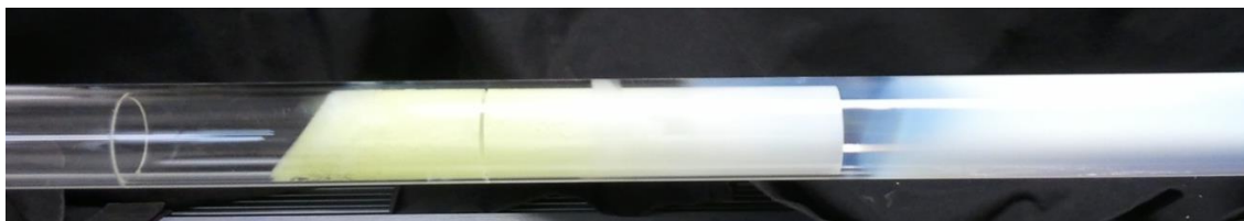
Figure 2.2: Photo of a typical collection tube after the thermal gradient sublimation of NPD.
