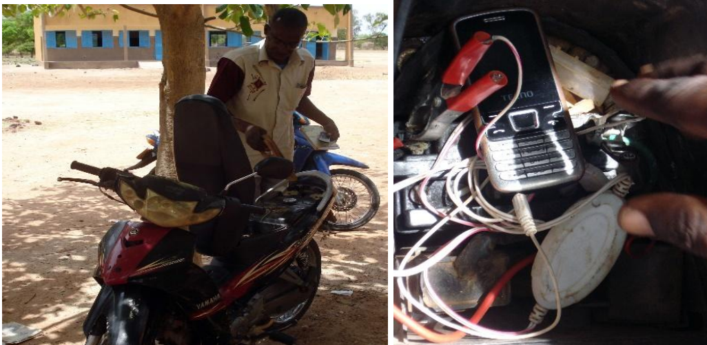
Figure 12. Departmental High School of Cassou-cell phone being charged through a motor cycle battery
