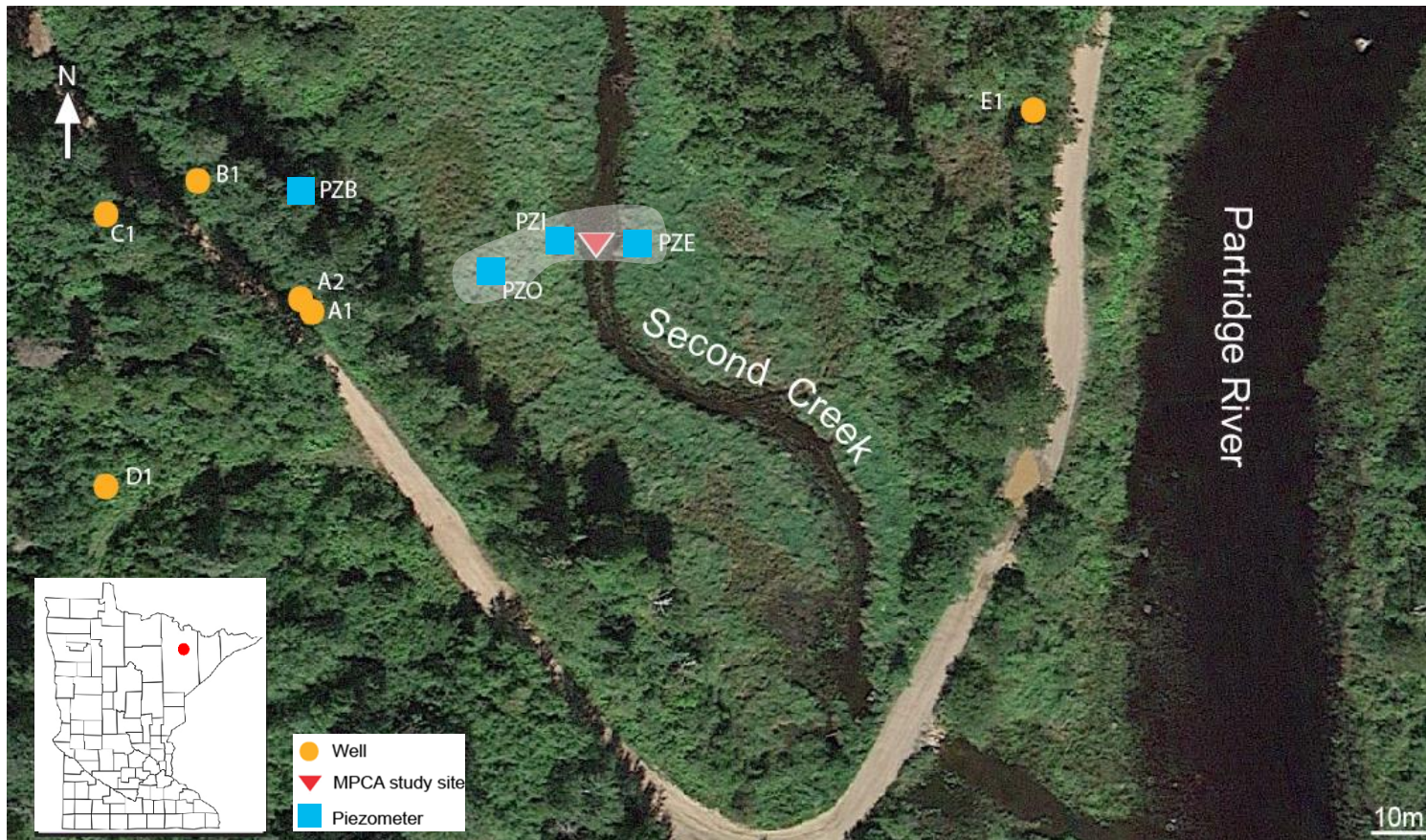
Figure 3. Location of groundwater wells (circles), piezometers (squares), and MPCA study site location (triangle) at Second Creek. Shaded area indicates area of focus of the temporary installations (temperature probes, seepage meters) and geochemical sampling locations.
