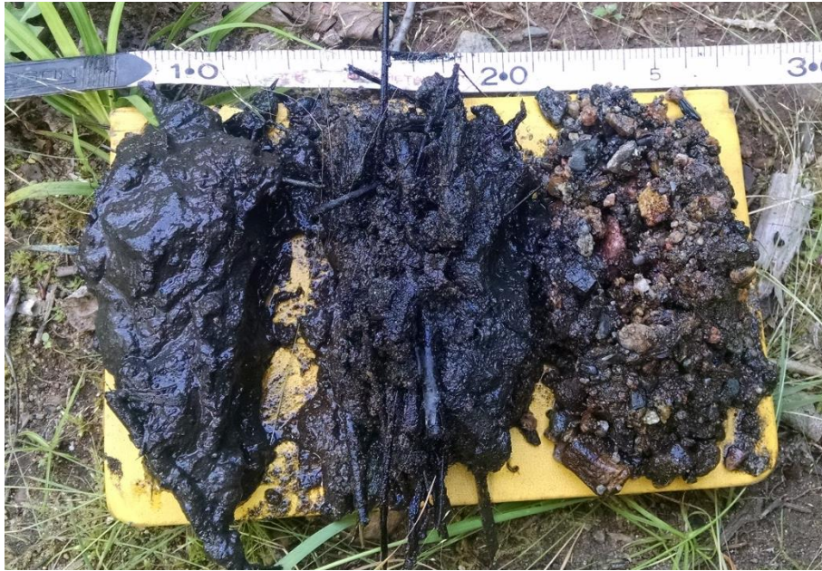
Figure 8. Sediment from the sediment water interface of the wetland (left) and two adjacent locations in main channel (center and right). Main channel sediment illustrated the high degree of sediment heterogeneity found laterally on the streambed of Second Creek.
