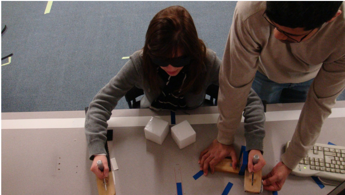
Figure 1. Bimanual manipulandum. A subject performing the contralateral matching task in a bimanual manipulandum with the examiner passively moving the non-dominant arm to the target position. All subjects were blindfolded with black opaque goggles during the contralateral matching task.
