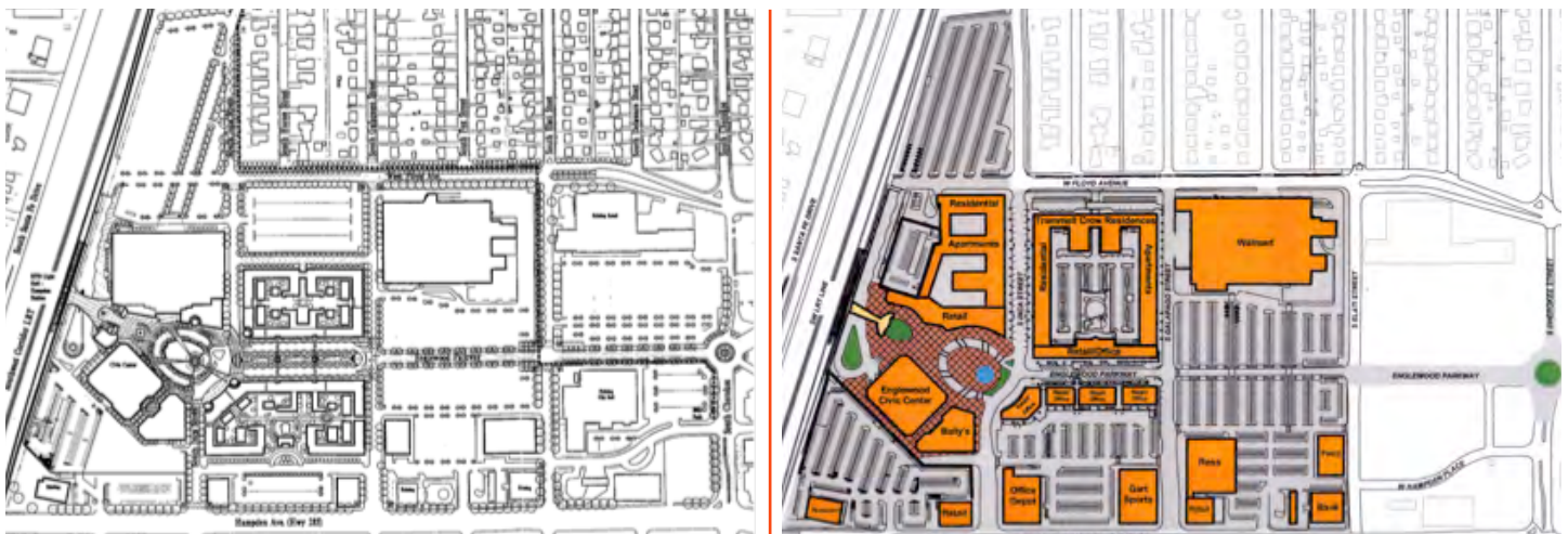
Figure 32. CityCenter Englewood as shown in the PUD plan (left) and as actually developed (right). The former Foley's building is on the far left of the site, adjacent to the station area and to the south and west of the plaza. Both images from Harold Stitt, via email, 2/13/13. PUD image from p. 55 of the original PUD plan.
