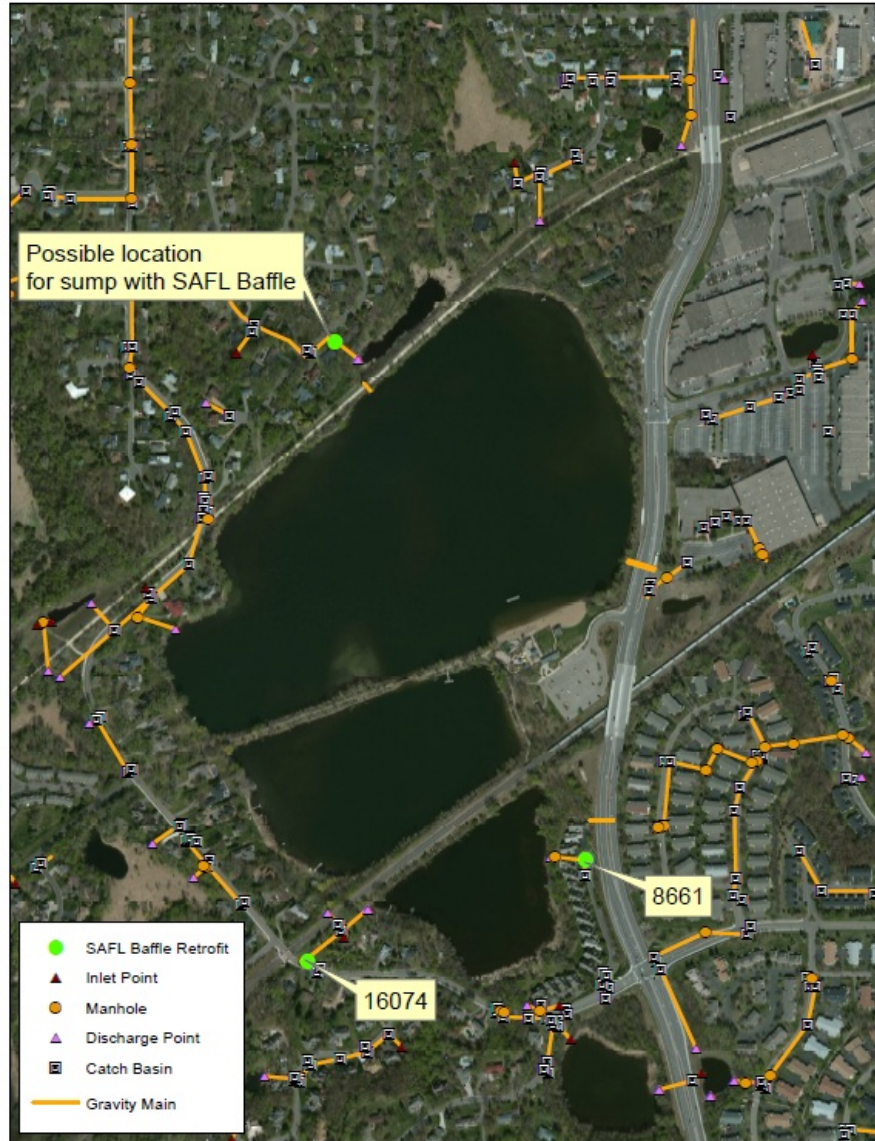
Figure 8: Current Sump Manholes Optimal for a SAFL Baffle Retrofit
