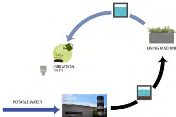
ABOVE: Diagram showing how water is recycled on-site with a Living Machine. Potable water is used for potable uses in the building, wastewater is treated and disinfected in the Living Machine to high-quality, non-potable standards. It is stored, then used for irrigation and toilets. The Living Machine could be incorporated into the mall atrium, or in a freestanding greenhouse.
