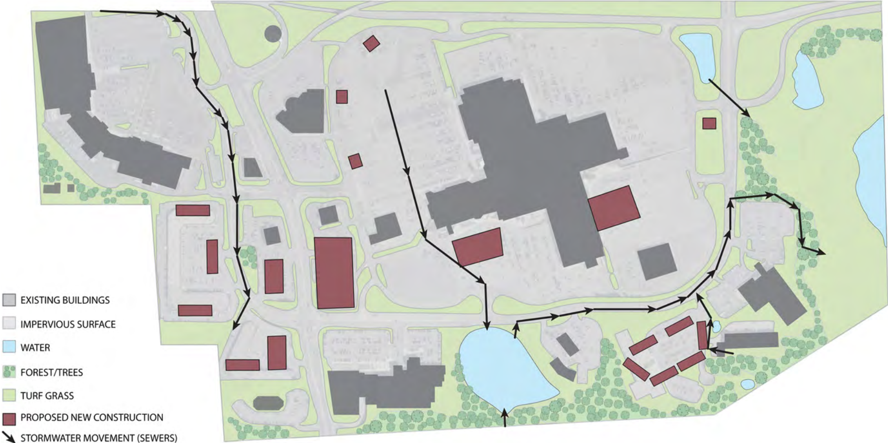
ABOVE : Diagram showing building footprints (existing and proposed), water bodies and existing ground cover. Also showing underground storm sewer drainage that conveys stormwater runoff into surface water bodies on site.
