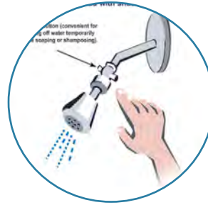
Use of low-flow fixtures can easily reduce potable water use by 30%
