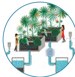
Treatment of Mall black+grey water using Living Machine gives additional reduction of 3% with overall reduction of site potable water of 55%
