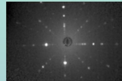
Figure 4: Laue X-Ray diffraction pattern for single crystal LSCO
