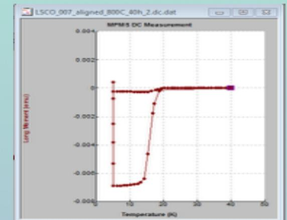
Figure 6: SQUID measurement for LSCO  $x = 0.07$ ; Superconducting transition temperature at  $\sim 17\text{K}$
