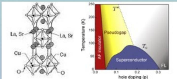
Figure 1: LSCO structure with  $\text{CuO}_2$  and  $\text{La},\text{Sr}$  planes
