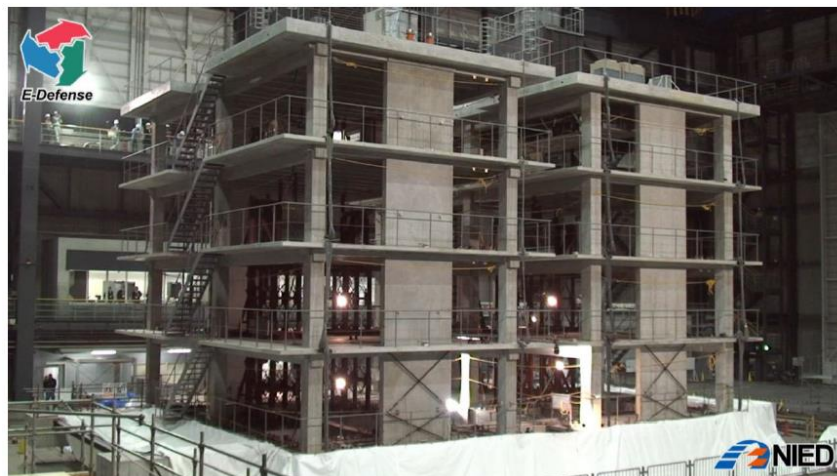
Fig. 2-37 E-defense shaking table tests (PT specimen on the left) (Tanyeri et al. 2013)
