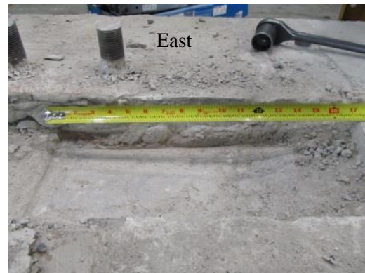
Fig. 6-31 Condition of the fiber grout layer beneath the west and the east wall corner
