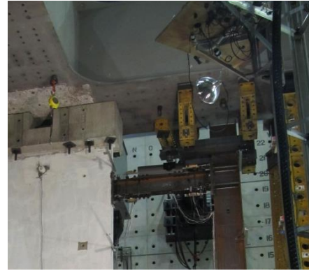
Fig. 3-85 Lateral support for steel columns
