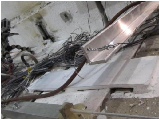
Fig. 7-107 Yield lines in the strap across plank-transverse beam connection at 4% drift in Phase 5
