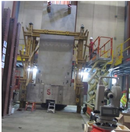
Fig. 3-66 Leveling the wall
