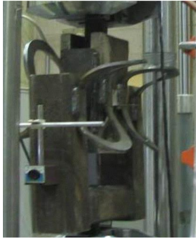
Fig. 9-8 Buckling of the O-connectors in the component test (Henry 2011)
