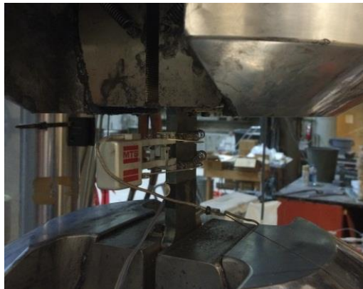
Fig. 3-150 Test setup for steel coupons
