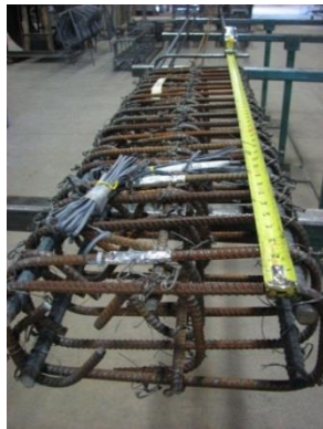
Fig. 3-57 Steel strain gages on the boundary element of the wall
