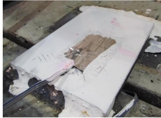
Fig. 7-106 Yield lines in the strap across plank-edge beam connection at 3% drift in Phase 5
