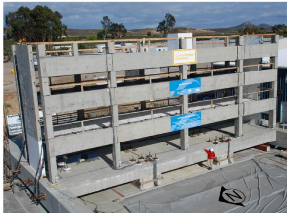
Fig. 2-33 Test setup of the shake table test (Schoettler 2010)
