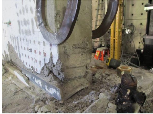
Fig. 9-5 Bending of the steel angle in the wall at the end of the test of PFS2
