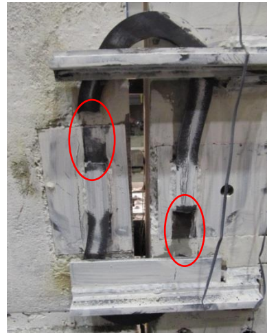
Fig. 7-94 Complete fracture of an O-connector at 5% drift in Phase 8
