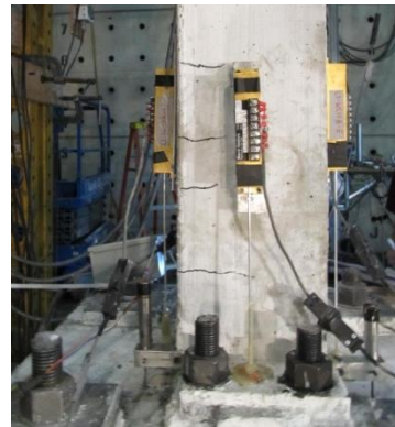
Fig. 7-120 Cracks in the fixed-base west edge column at 0.07% drift in Phase 3
