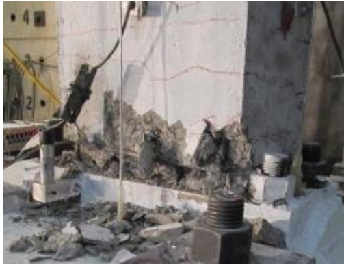
Fig. 7-127 Conditions of the west column after 5% drift in Phase 8
