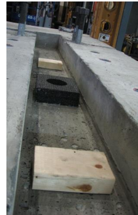
Fig. 3-50 Formed pocket in the base block
