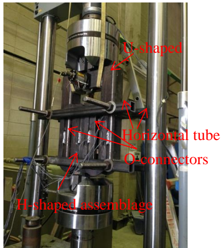
Fig. 2-15 Test setup for the O-connectors
