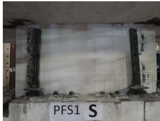
Fig. 6-60 Condition of the end columns (steel tubes) following the end of the test
