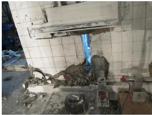
Fig. 8-24 Condition of the fiber grout beneath the west end column after 4% drift in Phase 5 of PFS2
