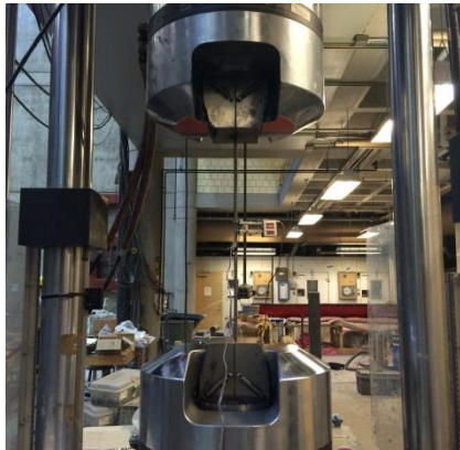
Fig. 3-148 Test setup for testing mild reinforcement
