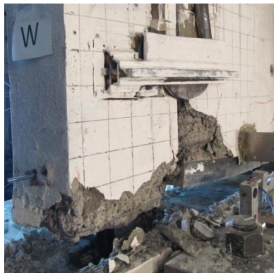
Fig. 7-59 West end column being picked up at 5% drift in Phase 10
