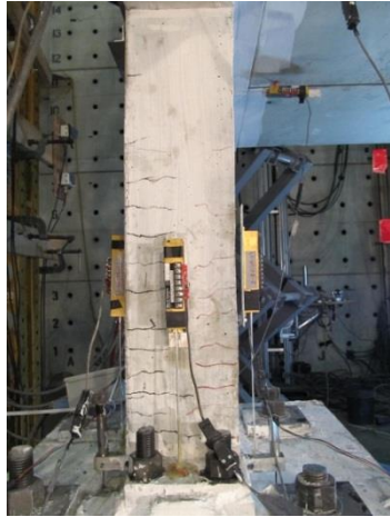
Fig. 7-121 Cracks distributed along the edge column at 1.5% drift in Phase 3
