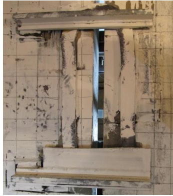
Fig. 7-91 Yield lines on the O-connector at 0.75% drift in Phase 1
