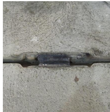
Fig. 7-108 Condition of the JVI Mini V connector after the test
