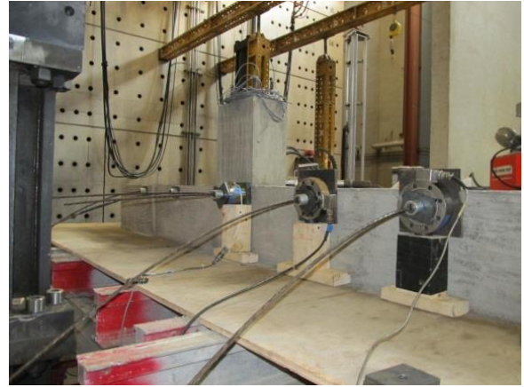
Fig. 3-79 Strands in longitudinal direction
