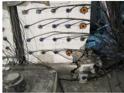
Fig. 8-25 Condition of the fiber grout beneath the east end column after 4% drift in Phase 5 of PFS2
