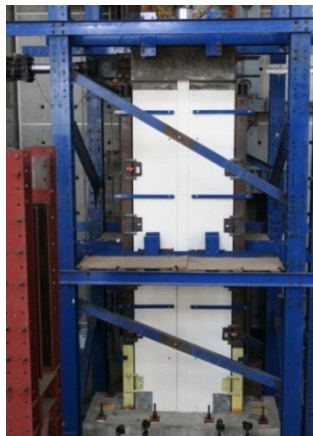
Fig. 2-17 Test setup of the PreWEC test in NCREE (Aaleti and Sritharan 2011)
