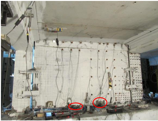
Fig. 8-17 Damage to the center of the wall base during the test of PFS2
