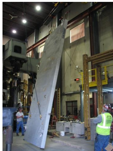
Fig. 3-65 Tilting up the wall
