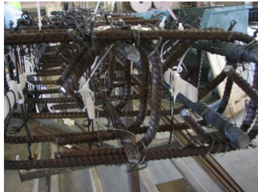
Fig. 3-58 Concrete strain gages in the boundary element of the wall
