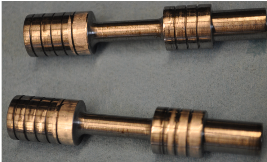
Figure 7.10: Picture of two mainstage spools after testing
