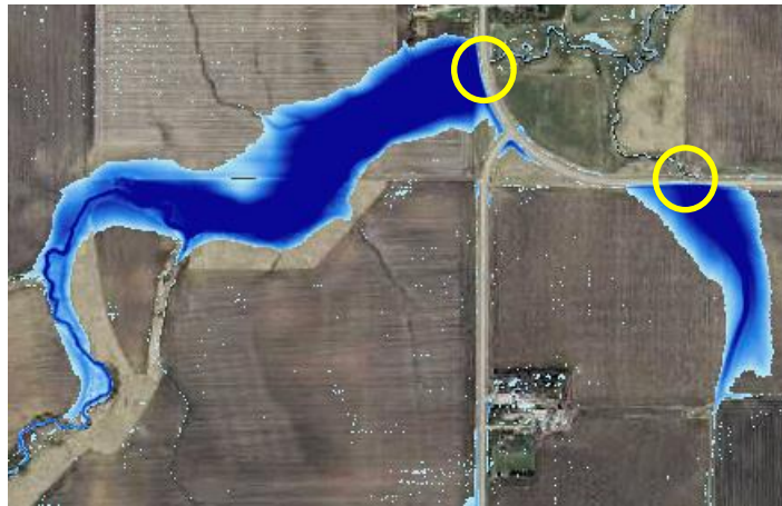
Figure 19. An example of how water ponds (in blue) behind road crossings when using a non-conditioned DEM. There are culverts present at both crossings (circled in yellow), though the DEM does not recognize culverts and sees the road as an obstruction – known as a digital dam.
