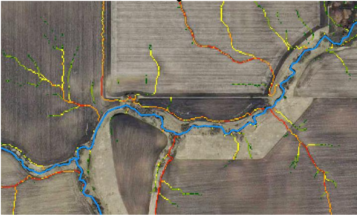
Figure 29. Spring-time acquired leaf-off imagery (top photo) clearly showing overland flow paths that can be used to match SPI signatures when establishing thresholds (bottom photo).
