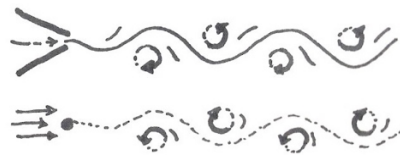
Figure 33. Paired, alternating vortex rotations in flowing media.
