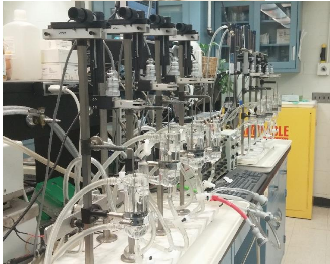
Figure 7: Muscle bath setup for contractile tests
