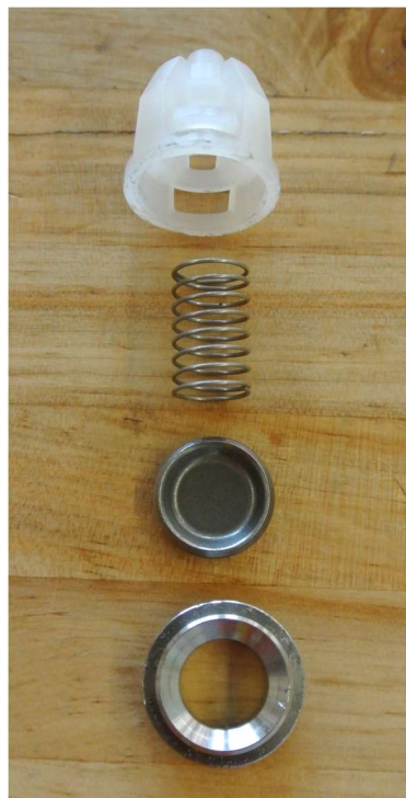
Figure 2.2. From top to bottom: disc valve housing, spring, disc, and seat
