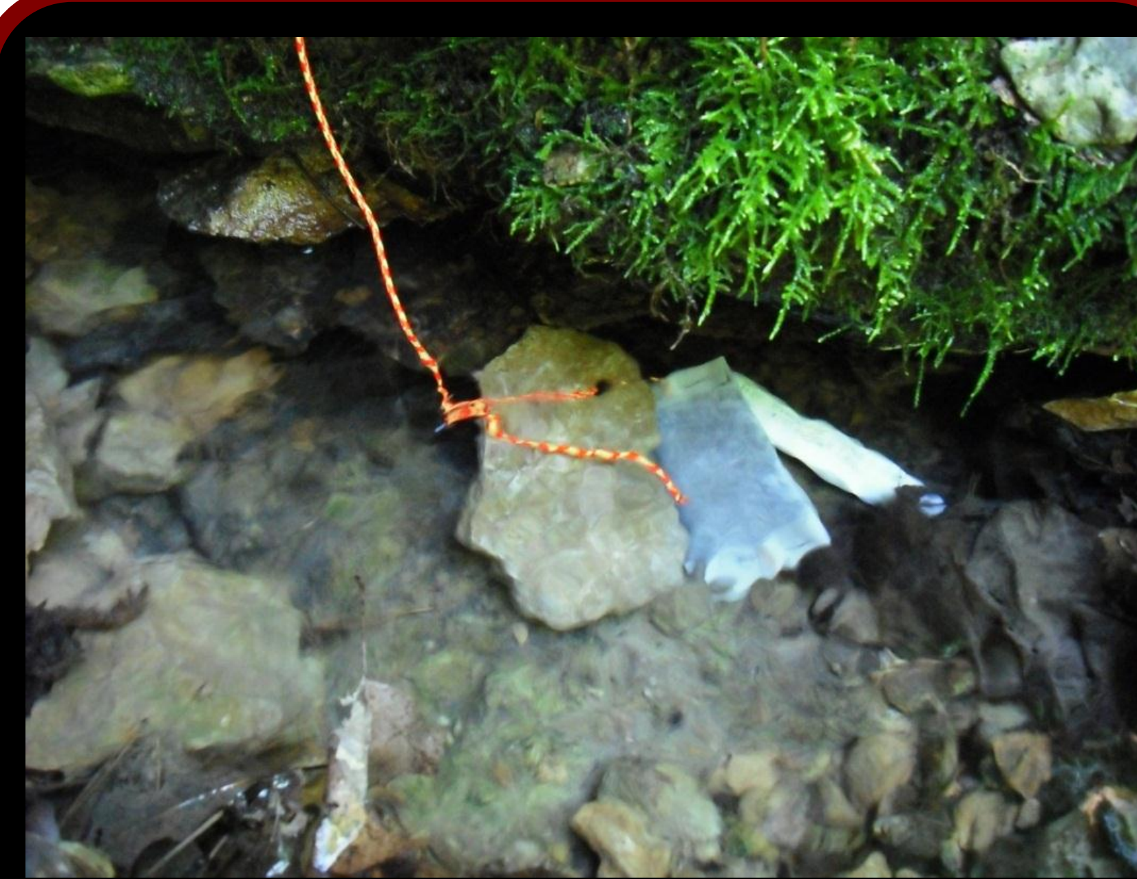
A bug detector contains activated charcoal, a material that's surface area is capable of trapping even the smallest amounts of dye molecules.
