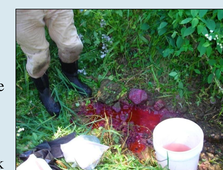
Right, pouring Rhodamine WT into a Kieffer Valley stream sink
