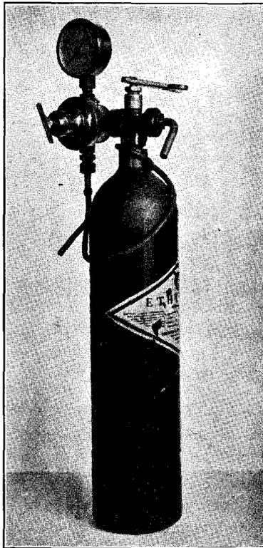
Fig. 5. Ethylene Tank with Expansion Valve and Nozzle
