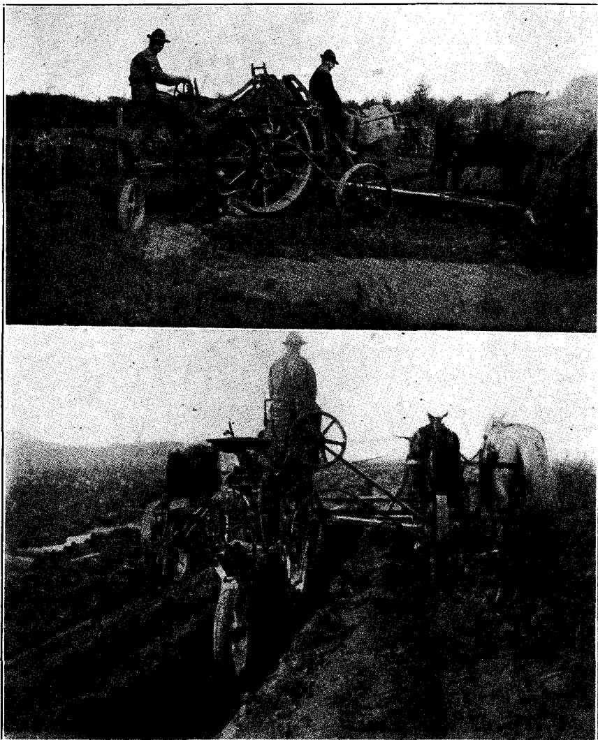
Fig. 32. Tile Ditcher, Light Traction Type
