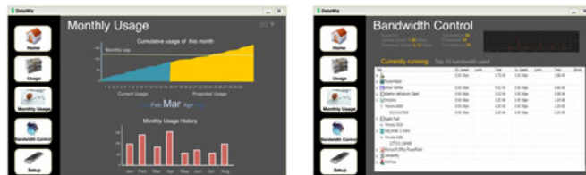
Fig. 2. Screenshots of the AMUSE prototype. Users can view their monthly usage and set bandwidth rates for individual applications.
