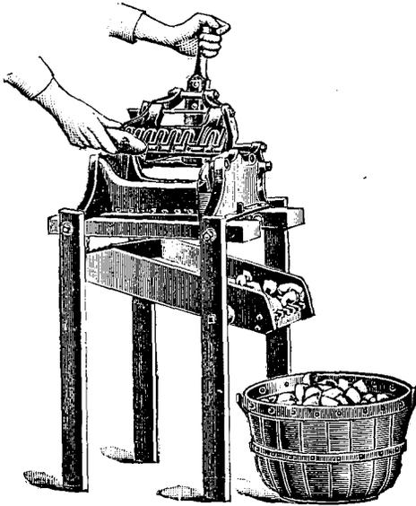
Fig. 213.—Aspinwall Potato Cutter.
