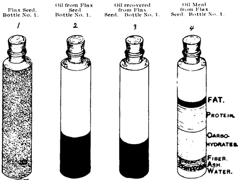
Figure 4. The oil and the oil meal obtained from a bottle of flax seed
