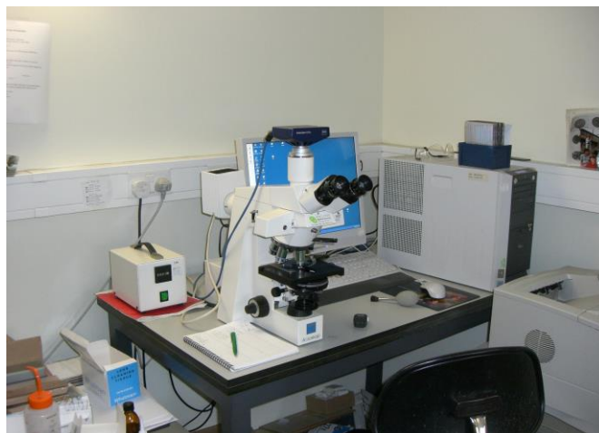
Figure 4-2. Optical microscope with mercury lamp attachment (FQM). The mercury lamp add-on allows for accurate fluorescence-quenching imaging
