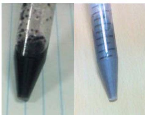
Figure 3-1. Appearance of GO reaction mixture a) – immediately after addition of \text{KMnO}_4 , and b) - after reaction completion
