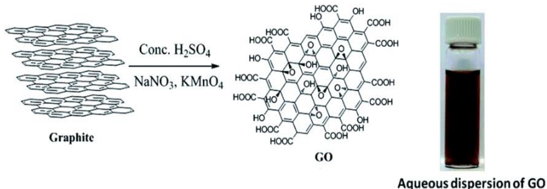
Figure 2-2. Schematic for the Hummers synthesis for GO, as depicted by Sharma et al.. (2014):
