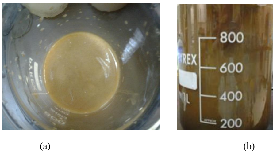
Figure 3-2. Appearance of a) aqueous graphite oxide at the end of the synthesis after adding hydrogen peroxide, and b)- graphene oxide (GO) at the end of the wash steps
