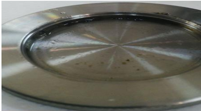
Figure B2-1. GO agglomerates at the cup bottom of the DHR3 DIN concentric cylinders at the end of a flow-sweep 1-100 1/s
