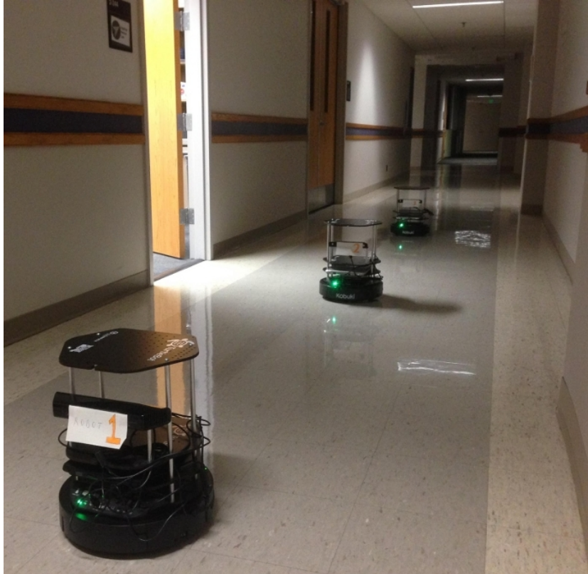
Figure 2.1: Turtlebot robots are in a patrol mission along the corridor following an optimal solution generated by our MCTS-UC approach. The robots are programmed by using ROS (Robotic Operating System) framework. We firstly map the corridor by creating a 2-D occupancy grid by using a particle filter based SLAM approach. Using this map, we developed a mission controller for patrolling that is built on top of ROS navigation and localization stacks.
