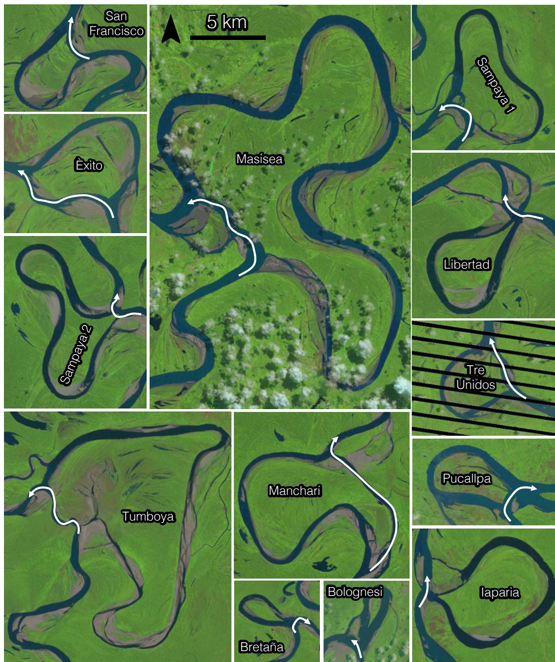
Figure 5.1: Thirteen cutoff events along the Ucayali River are shown midway through the cutoff process and at low flow. Cutoff channels and flow directions are denoted by white arrows. The north arrow and scale bar apply to all images.
