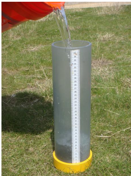
a) Place the permeameter clear tube on the secured base and use gentle force to fully insert clear tube into the base, level it evenly and fill with water.
