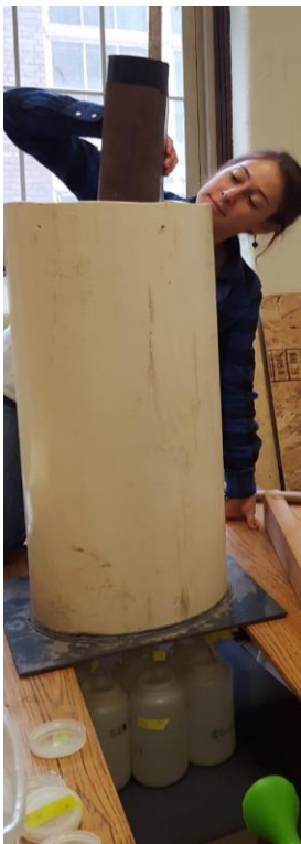
Figure 16. Soil Core with Infiltrimeter (left) and Soil Core Bottom with Bottles (right)
