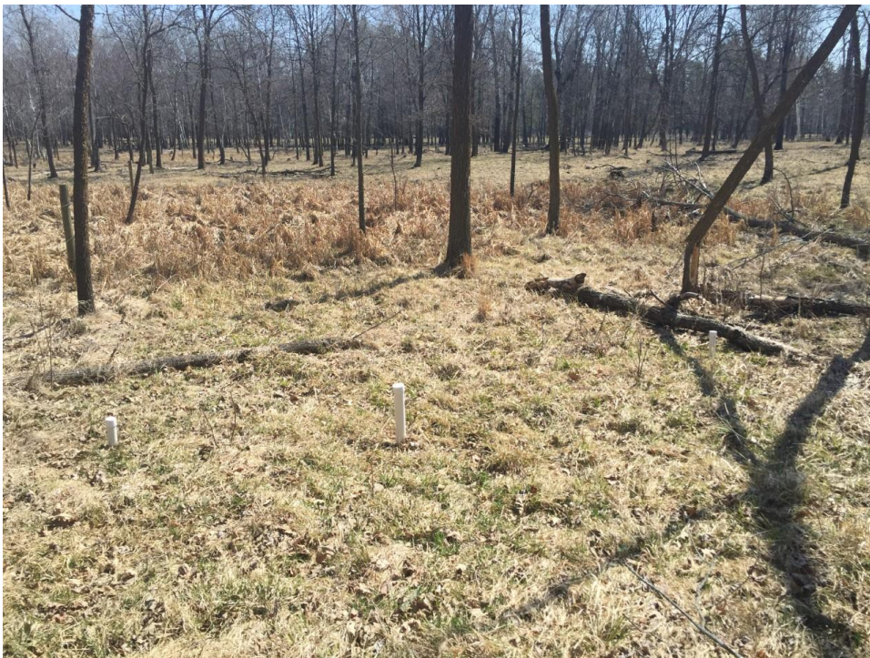
Figure 12. Vadose Zone Access Tubes Located in Caughey's Traditional Forest Paddock
