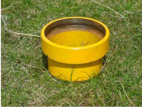
(a) Place the permeameter base in an area that permeability ( K_{sat} ) is to be measured.
