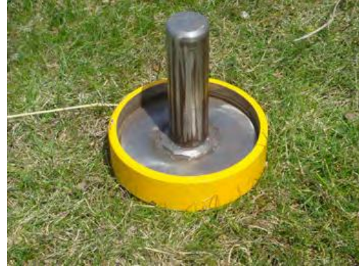
(b) Place ring weight inside the base and use a hammer to force the permeameter base into the soil up to the bottom of upper ring.
