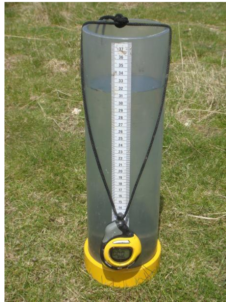
b) Wait for water surface to stabilize, read water level and start timing. Continue to read water level and time.
