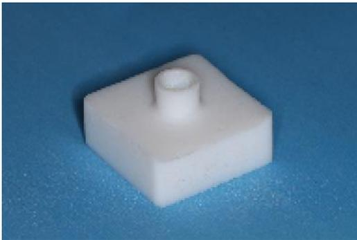
**Figure 2:** Teflon mold
