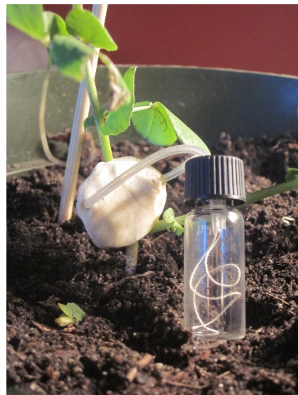
Figure 3.6 Tubing is threaded through hole in cap with septa, and thread reaches bottom of vial.
