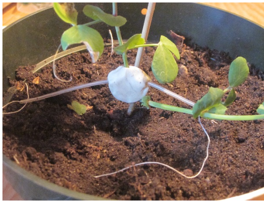
Figure 3.5 Plasticine is fully molded around tubing and stem.
