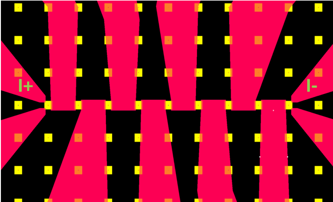
Figure 3.2: A close-up cartoon of the sample geometry. Pink areas represent the W/Au contacts, and yellow areas represent the magnetic dots. With this geometry, current can be sourced through the ends on the contacts marked I+ and I-, and then any other pair of contacts can be chosen as voltage contacts to measure any combination of adjacent dots simultaneously.
