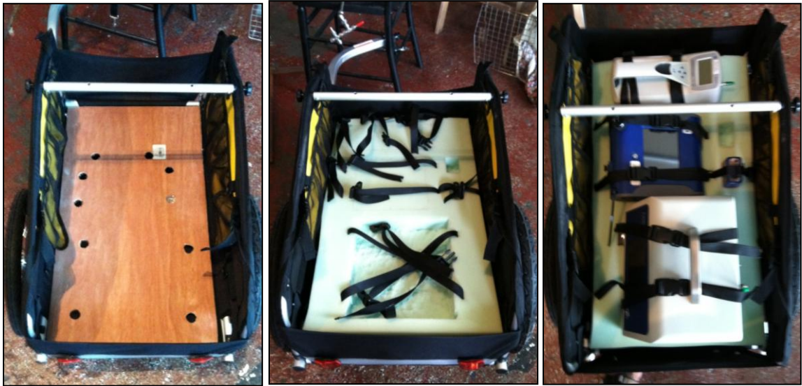
Figure 2.1 Three stages of installation of the padded mounting system for the Burley Nomad Cargo trailer.
