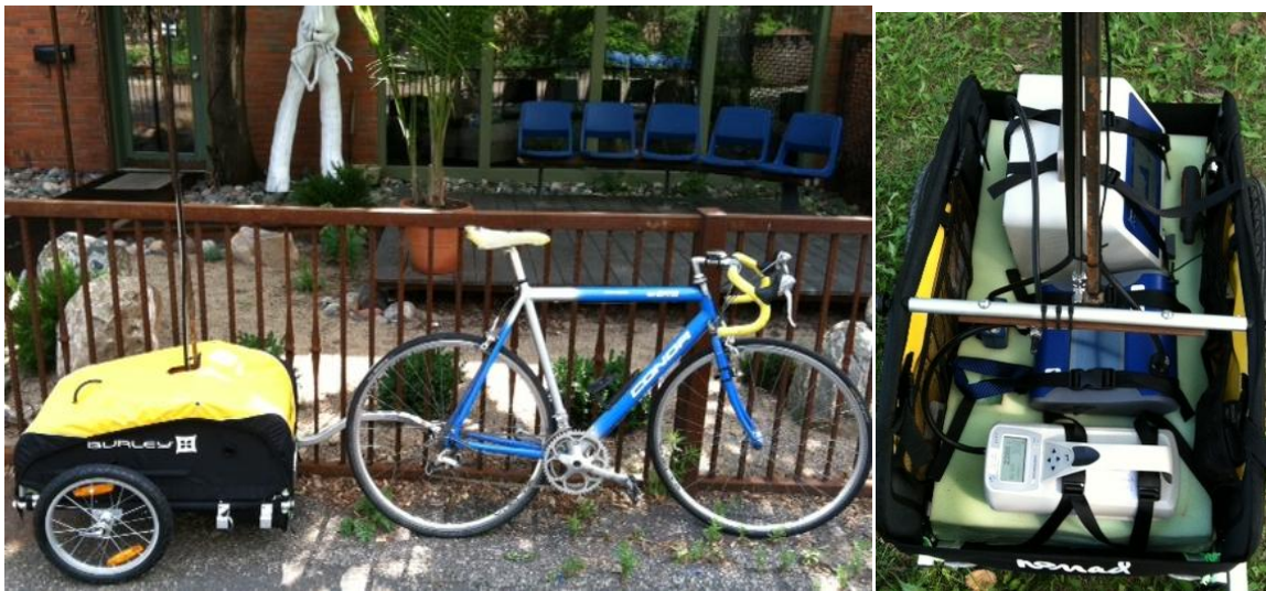
Figure 2.3 Final mobile sampling bicycle trailer configuration.
