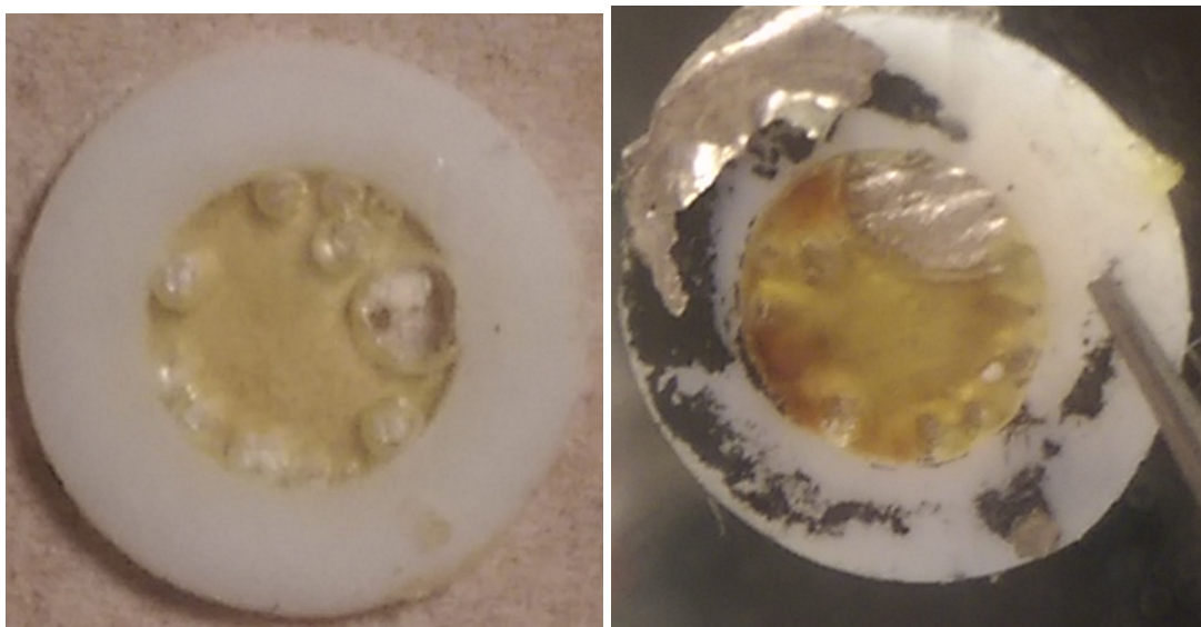
Figure 4.26: Images of sample (a) before and (b) after cycling. The silver foil is lithium metal, and the white washer is PTFE. The black marks on the PTFE suggest that the lithium metal reacted with the PTFE.
