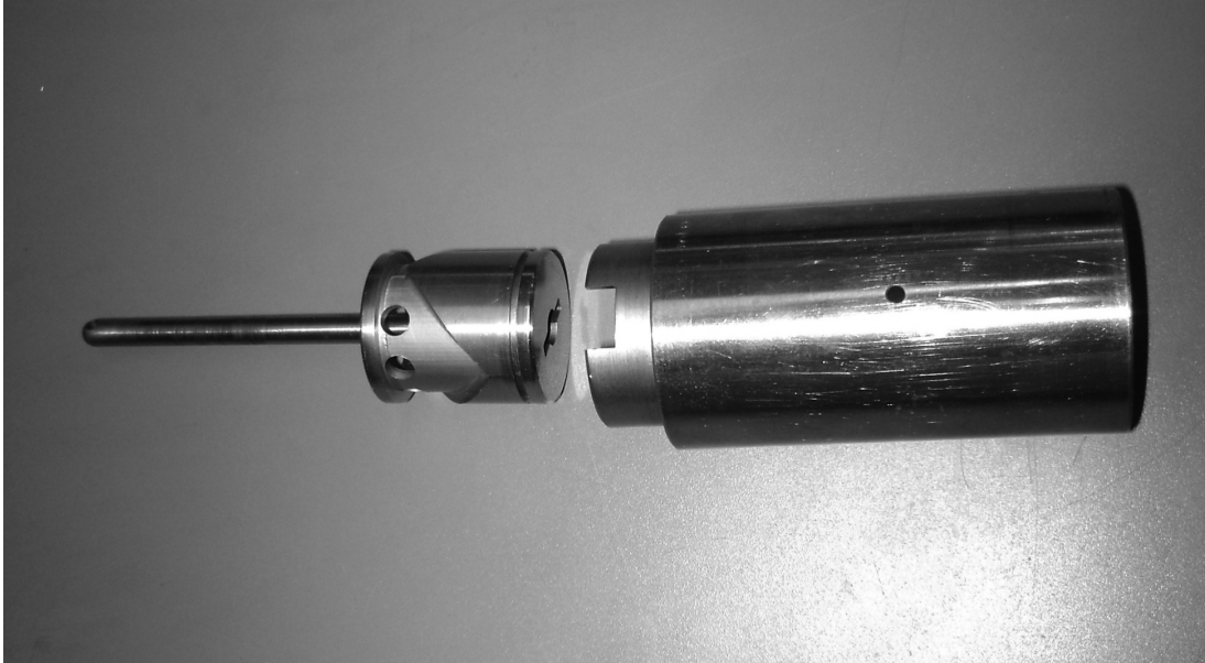
Figure 1.5: Generation 2 helical rotary on/off valve spool and sleeve designed by Adrian Durand at the University of Minnesota (2006).
