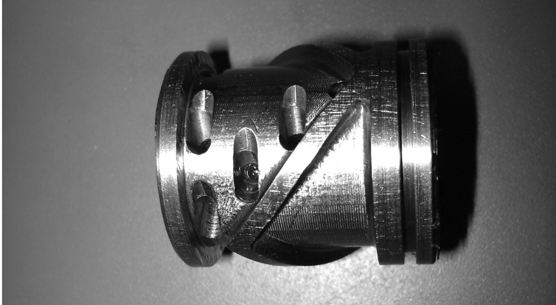
Figure 1.6: Generation 2.5 helical rotary on/off valve spool modified to demonstrate self-spinning functionality. Self-spinning is achieved by reversing the flow path of the generation 2 valve such that the inlet port of the valve is tangential to its axis of revolution.
