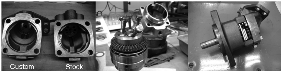
Figure 3.29: Left: Custom 4-way P/M housing compared to stock housing. Center: Fixed displacement bent axis P/M disassembled to replace housing and insure correct timing. Right: Fully re-assembled P/M with custom housing installed.
