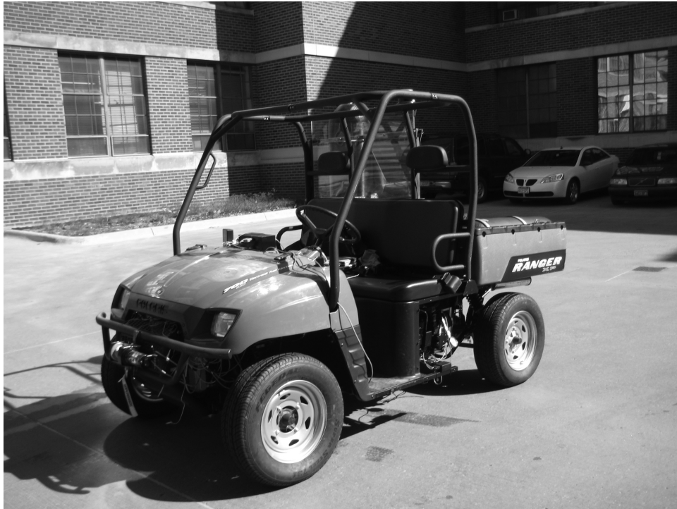
Figure 3.1: Polaris Ranger hydraulic hybrid passenger vehicle test bed at the University of Minnesota based on an input coupled power-split drive train.
