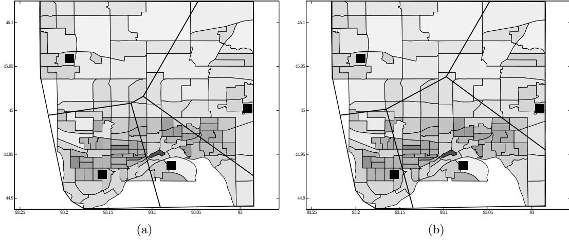
Figure 4.6: Two power diagram partitions of the service region \mathcal{R} . The weight associated with the bottom right sub-region is larger in (4.6a) than in (4.6b).
