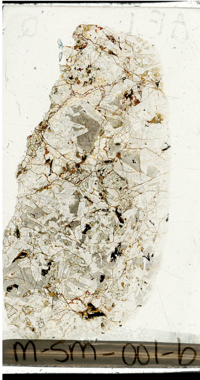
Figure 3-5. Thin section scan of thin section M-SM-001-b. Note absence of rust colored coatings around outer edge. Slide dimensions = 27 × 46 mm.
