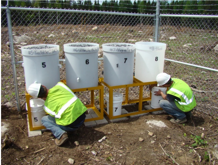
Figure 1-5. Photo of barrel tests constructed on site at Mesaba in June, 2013. Small lower buckets are used to collect water (atmospheric precipitation) that drains through the crushed rock contained in the barrels.
