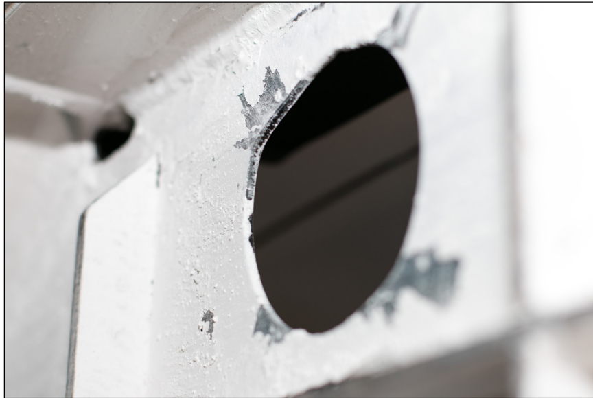
Figure 5-6: Test 2 – Out-of-plane displacements in CT subpanel
