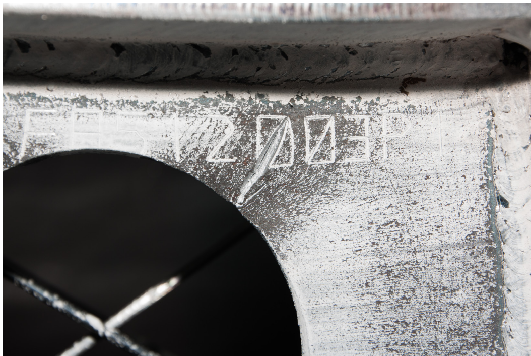
Figure 5-39: Test 7: Crack formed at the indented part number defect (t=25.00)
