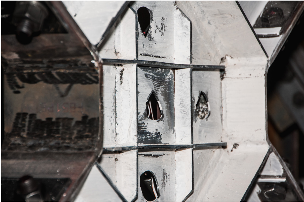
Figure 5-13: Test 3 – Out-of-plane displacements in the web at t=20.75
