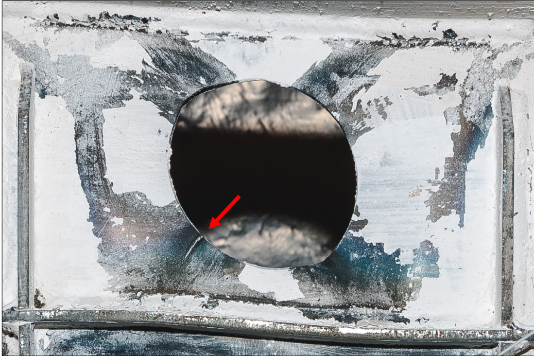
Figure 5-8: First observed damage in CT subpanel for Test 2
