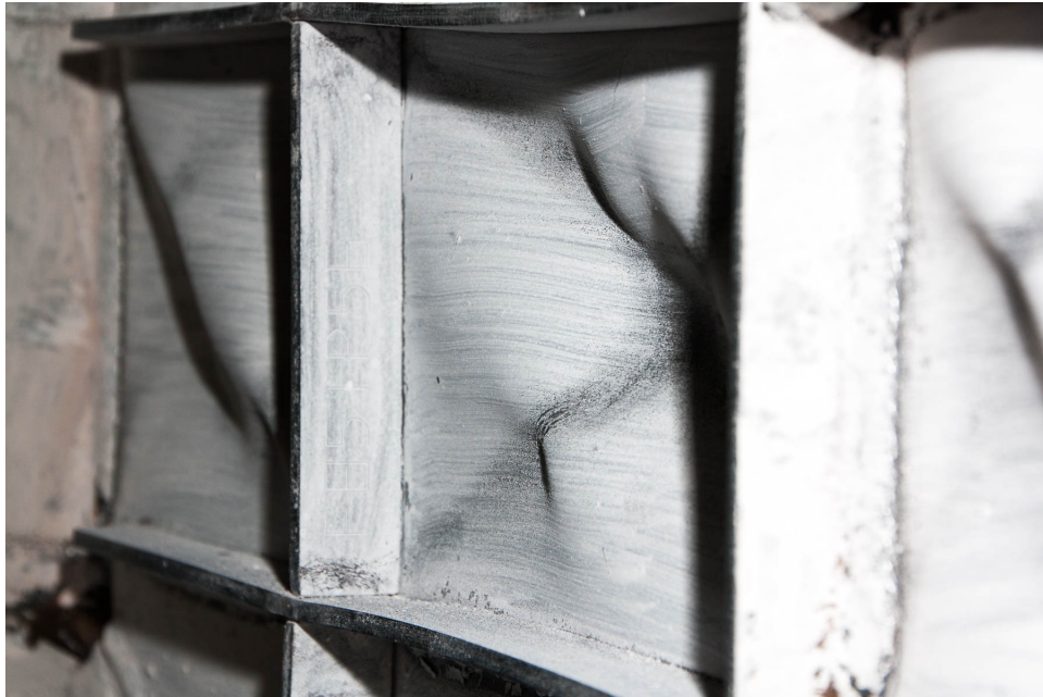
Figure 5-51: First crack forming on CM subpanel in test 10
