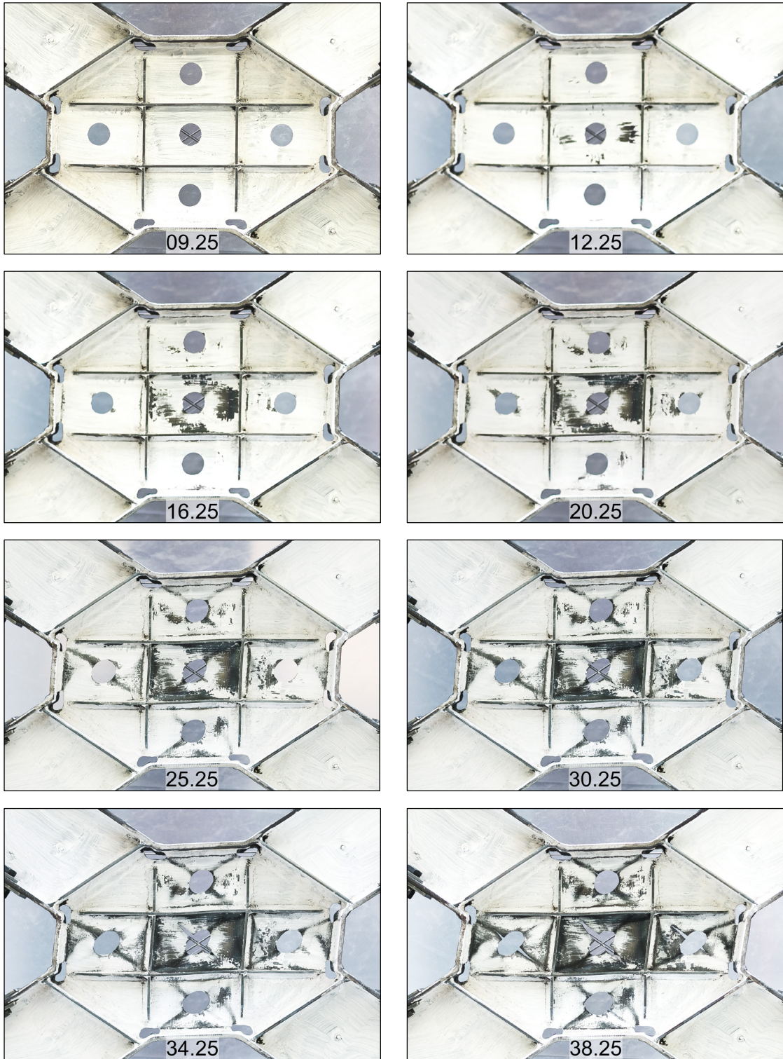
Figure 5-12: Test 3: Yielding and damage evolution
